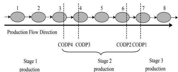
Fig.5 Abstract Liner Diagram of Turbines Production
