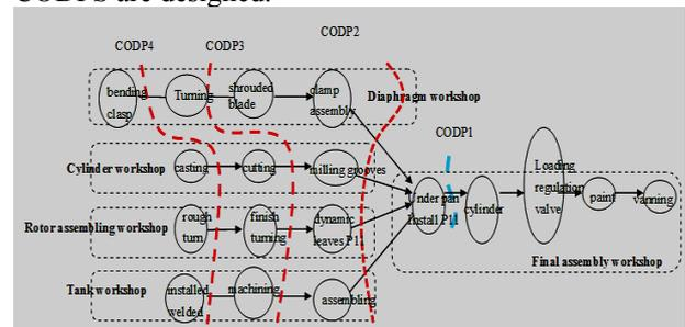
Fig.4 Multi-CODPS Mass Customization Production System of Turbine Machine
