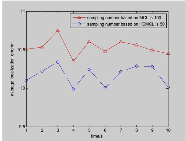
Fig.3 The Effects of Sampling number on the MCL and HDMCL Algorithms
