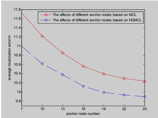
Fig.4 The Influence of Anchor Node Density on the Node Location
