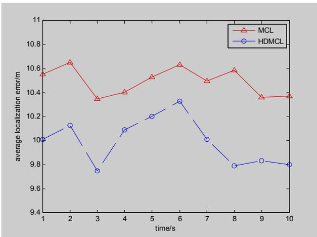
Fig.2 Comparison Chart of Location Accuracy Based on MCL Algorithm and HDMCL Algorithm
