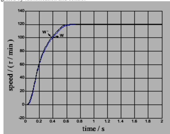
Fig.9(a)) Motor speed waveform in 120r/min and no load start
