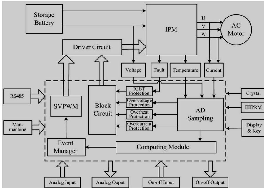
Fig.8 Frequency control system structure integrated by identification and control
