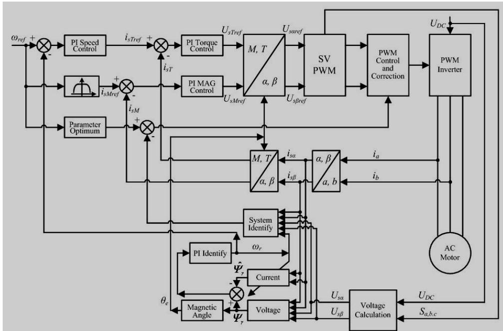
Fig.6 Working process with load identification and adaptive frequency control
