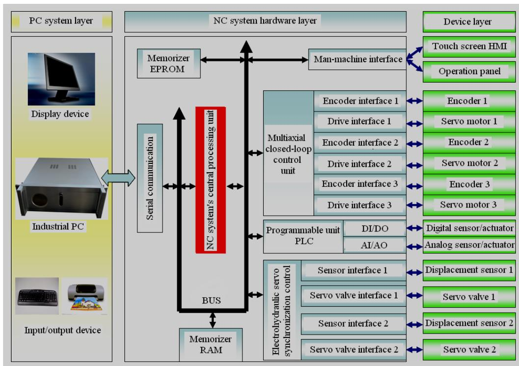
Fig.10 The CNC system based on the real-time error compensation
