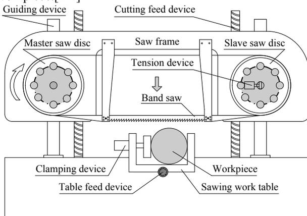
Fig.1 Composition of CNC cutting equipment
