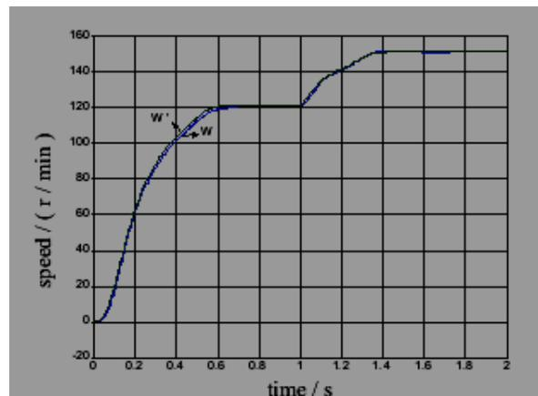
Fig. 9(b) Motor speed waveform from 120r/min to 150r/min at 1s
