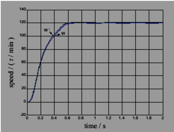
Fig.9(c) Motor speed waveform from 0 to 15Nm at 0.8s in the given speed 120r/min
