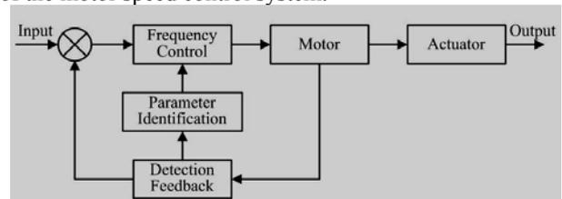
Fig.5 Block diagram of identification and adaptive frequency control system
