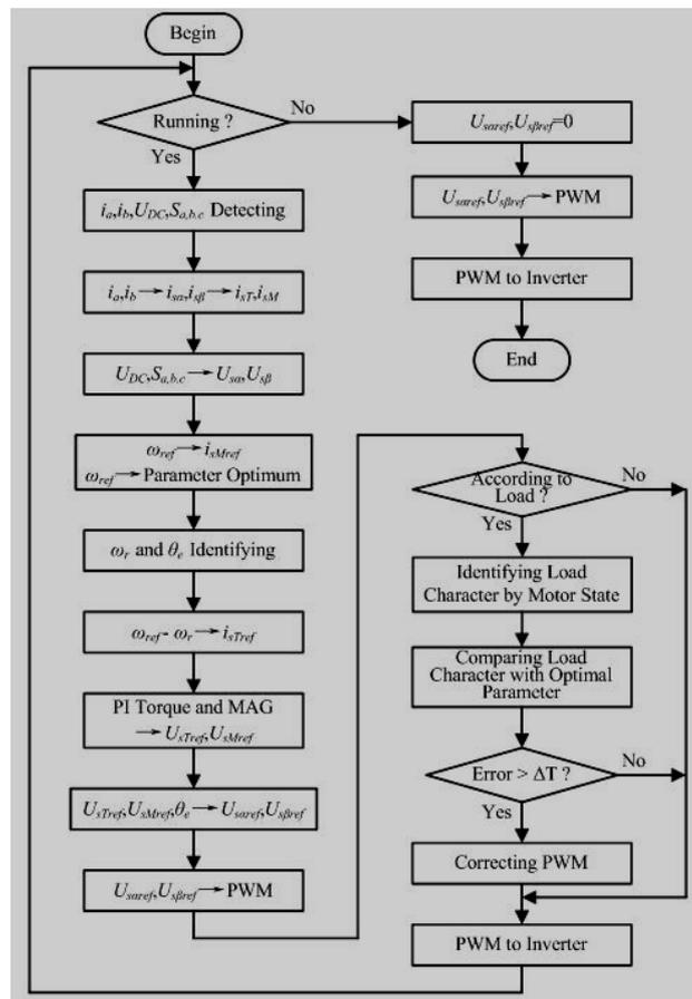
Fig.7 Software flow of the inverter control system
