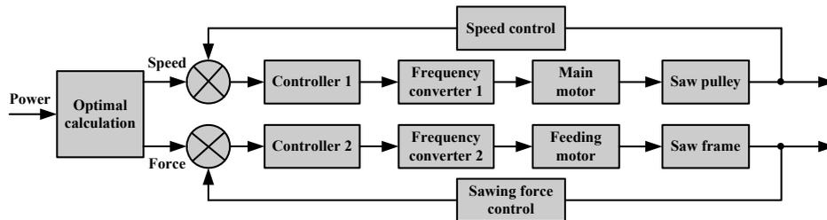
Fig.2 Sawing control model of constant power
