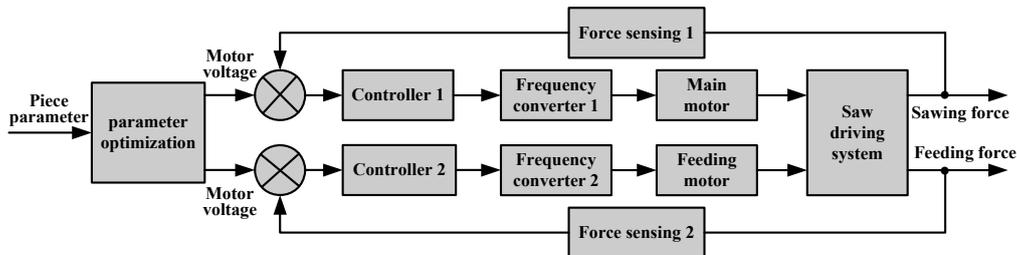
Fig.3 Control model of the equipment's constant force
