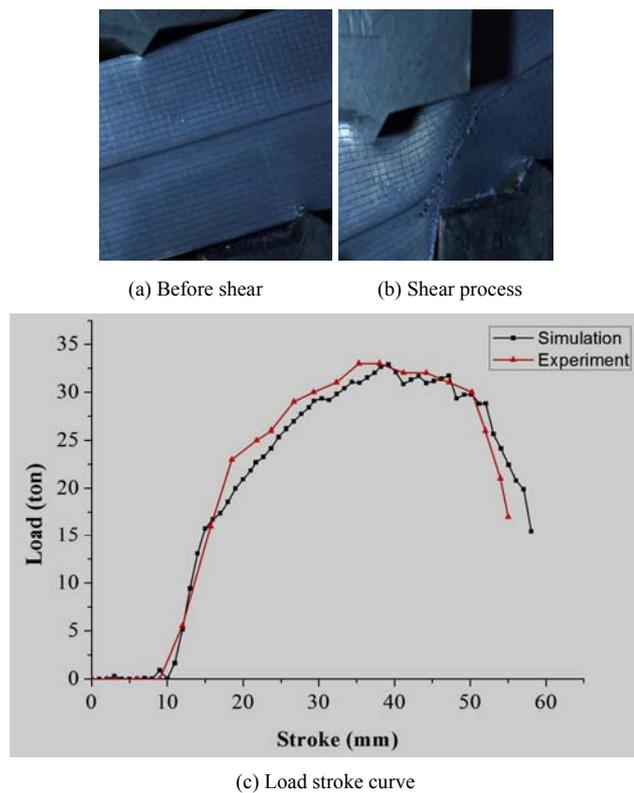
Figure 5. High temperature, high speed shear on thick plates.
