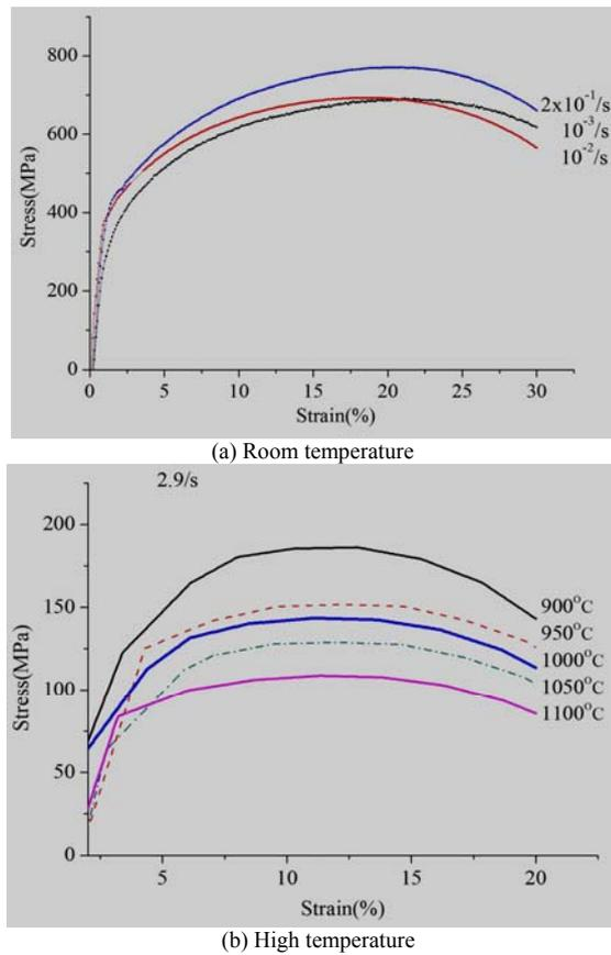
Figure 1. Gleeble tensile curves.
