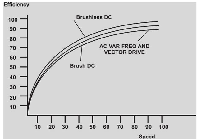
Figure 12. Efficiency vs. speed graph.
