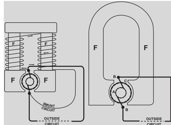
Figure 1. Self-excited shunt DC motor
