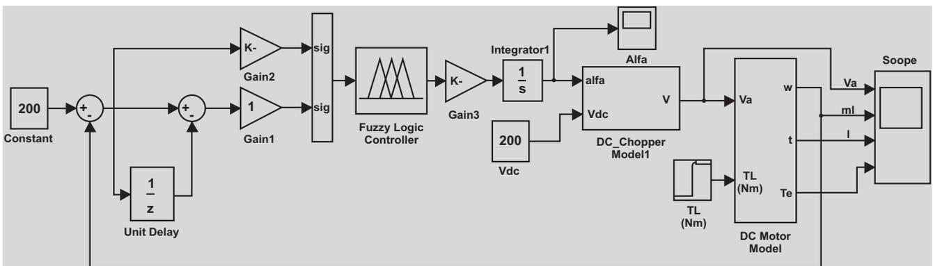
Figure 10. Fuzzy model for the motor.
