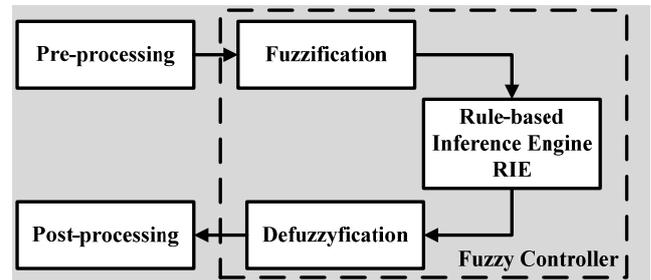
Figure 6. Block diagram of fuzzy logical control.
