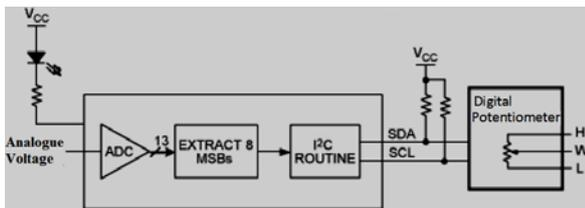
Fig.5 The Basic Circuit Schematic Diagram Of The Controlled Digital Potentiometer
