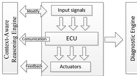
Fig.1 The Composition of the Simulation Diagnostic System
