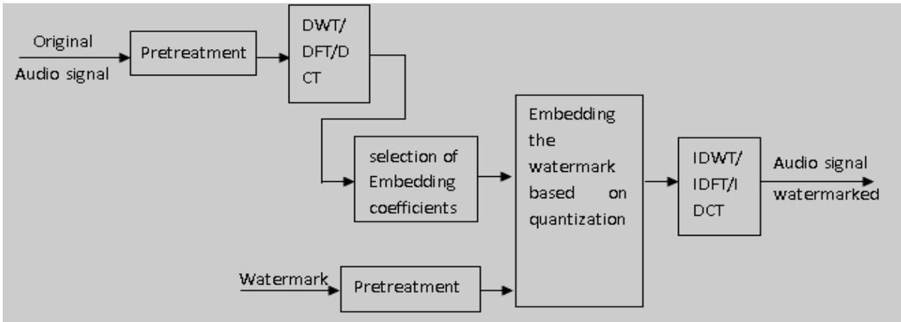
Fig.2 Embedding Watermark Algorithm Diagram
