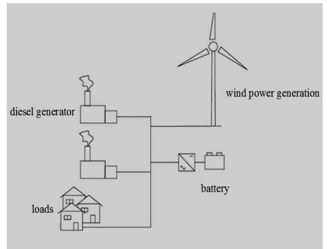
Fig. 2. Hybrid energy power system structure
