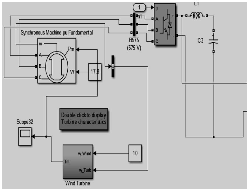
Fig. 3. Simulation of Wind Power Generation
