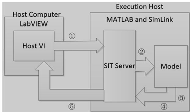
Fig. 1. Interface between LabVIEW and Simulink.
