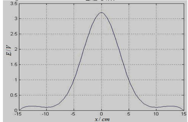
Figure 4. The relation between coils induced electromotive force and horizontal distance of wires.
