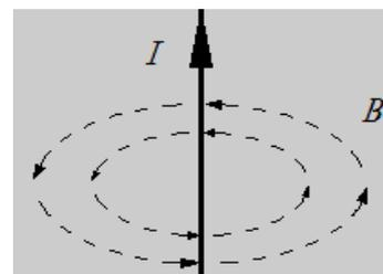
Figure 1. Distribution of the magnetic field intensity around straight current-carrying wires
