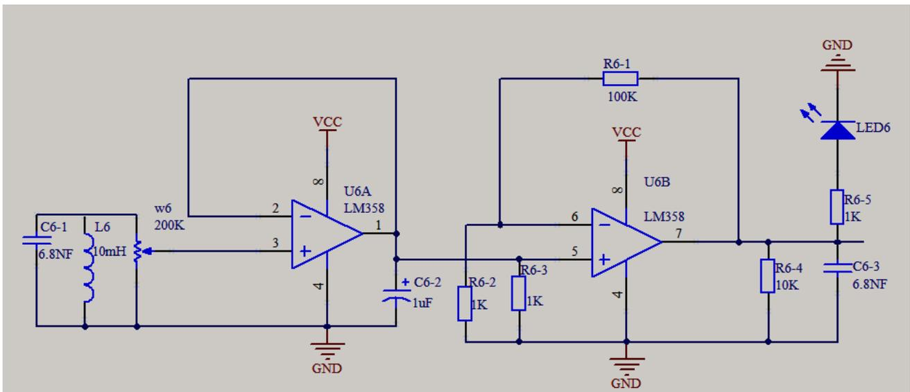
Figure 6. The amplify circuit of sensors.
