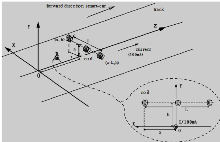
Figure 3. Lay-out modes of sensor coils.
