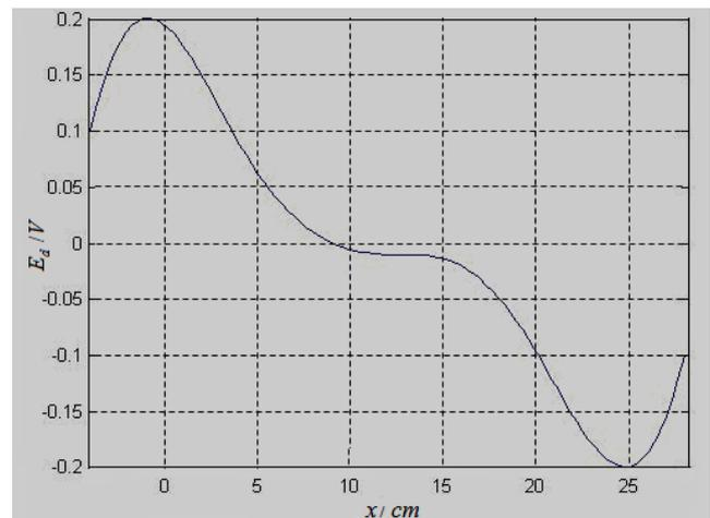
Figure 5. The relation between difference values of coils induced electromotive force and horizontal distance of wires
