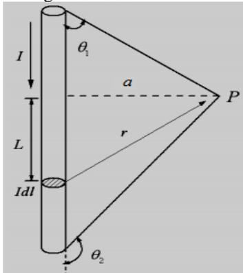
Figure 2. Magnetic field intensity calculating of straight current-carrying wires.
