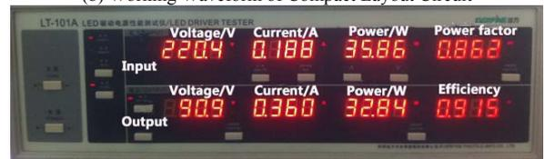
(c) Experimental Parameters of Optimized Layout Circuit
