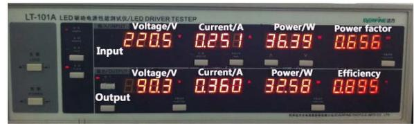
(a) Experimental Parameters of Compact Layout Circuit
