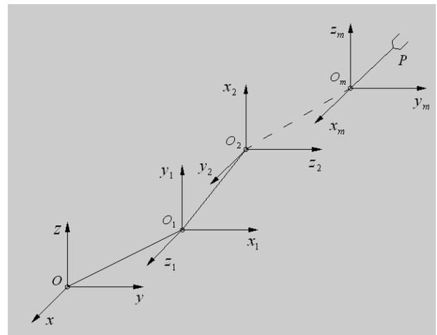
Fig.1 Homogeneous transformation mapping of moving element
