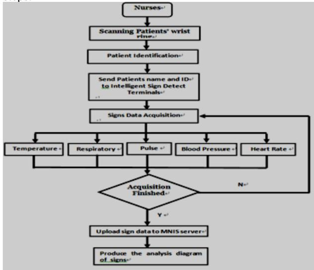
Fig.8 The work flow of MNIS
