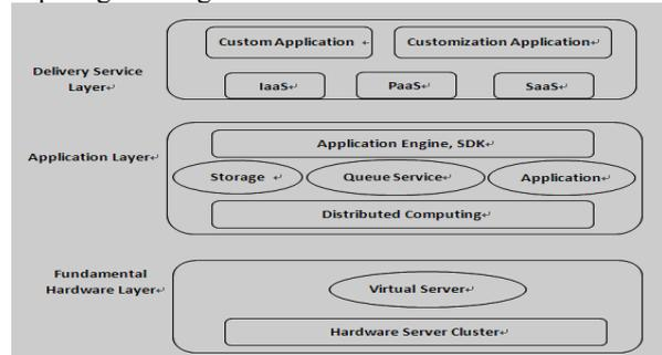
Fig.2 The architecture of cloud computing
