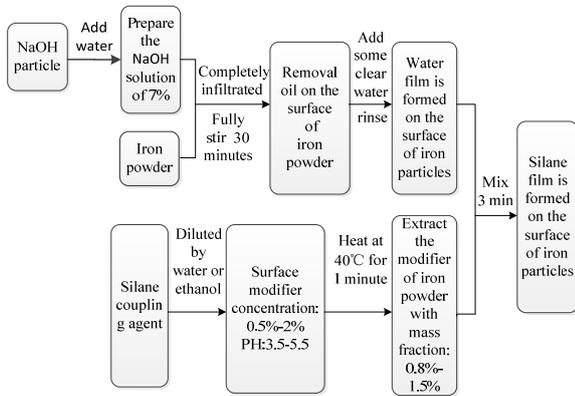
Fig.7 Fe Surface Modification Process
