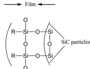
Fig.6 The Surface Chemical Bonding Model of SiC Particles After The Surface Modification Using Silane Coupling Agent
