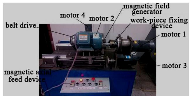
Fig.8 Experimental Device
