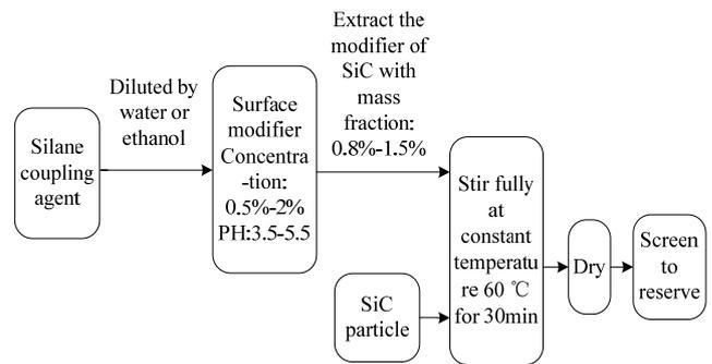
Fig.5 SiC Surface Modification Treatment Process
