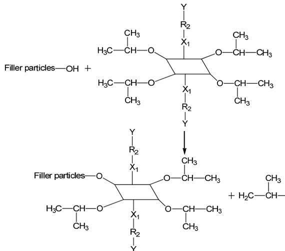
Fig.3 Reaction Mechanism Between Titanate Coupling and Filler Particles
