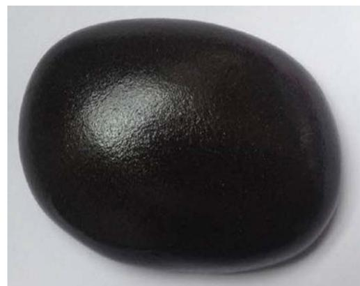
Fig.1 Viscoelastic Magnetic Abrasive Tools
