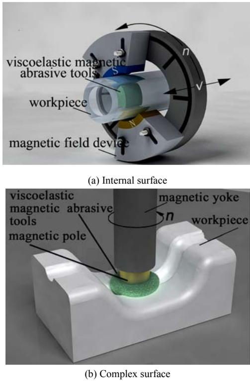
Fig.2. Viscoelastic Magnetic Abrasives Finishing Schematic Diagram
