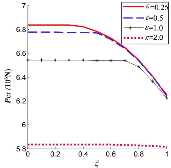
Fig.5 The Curve of  $P_{cr}-\xi$  With Eccentricity
