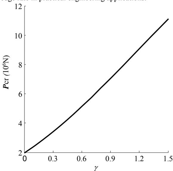
Fig.7 The Curve of  $P_{cr}-\gamma$  With Crack Length
