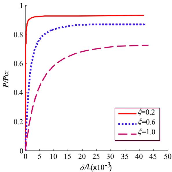
Fig.9 The Curve of Load-Displacement With Crack Length
