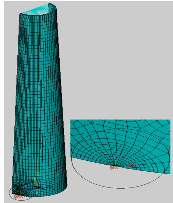
Fig.3 Finite Element Model of Thin Walled ShuttleCylinders Structure
