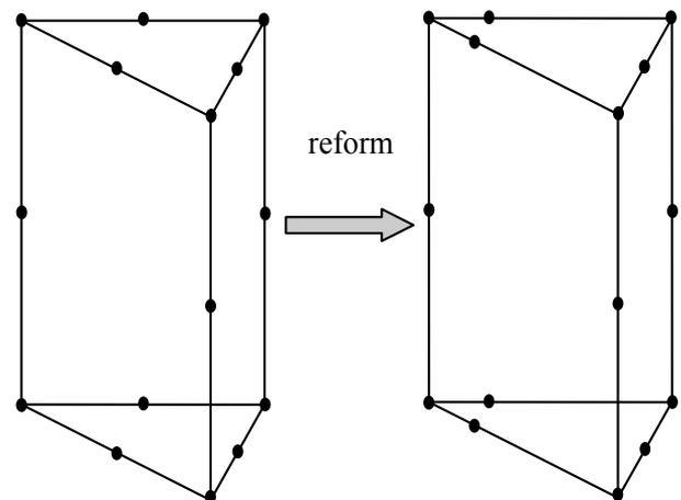
Fig.4 The Element of Crack Front About Before And After The Improvement
