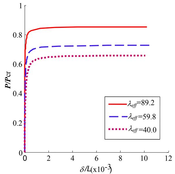
Fig.10 The Curve of Load-Displacement With Slenderness Ratio
