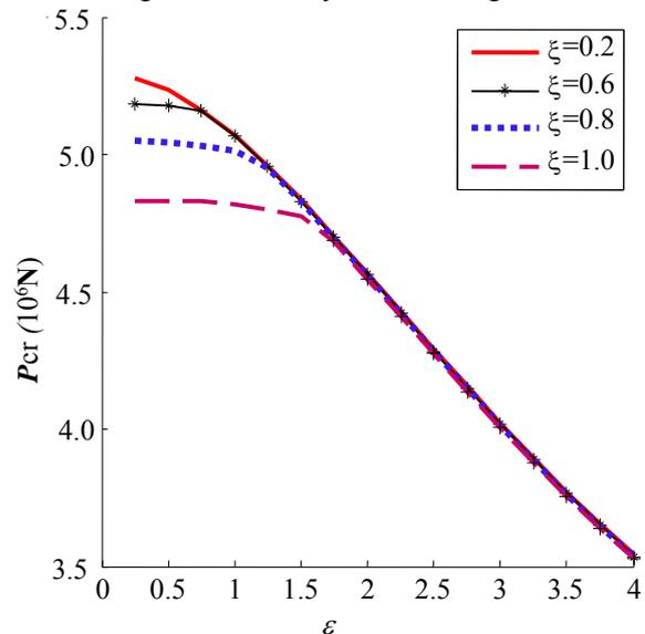
Fig.6 The Curve of  $P_{cr}-\varepsilon$  With Crack Length
