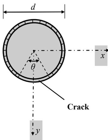
Fig.2 Cross Section With Crack
