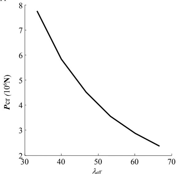
Fig.8 The Curve of  $P_{cr}-\lambda_{eff}$  With Crack Length
