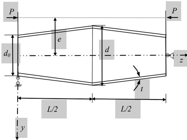
Fig.1 Thin-Walled Shuttle Cylinders Structure With Crack Under Eccentric Compression
