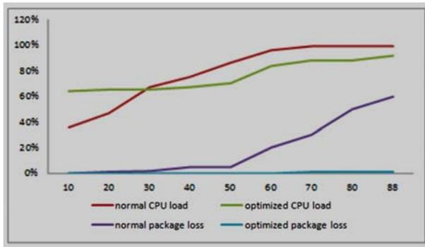
Fig. (4). Packet Loss Rate, CPU Load and Sensor Node Curve
