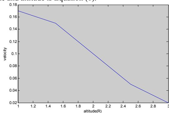
Figure 4. Velocity of ground effect on rotor plane at different altitudes
