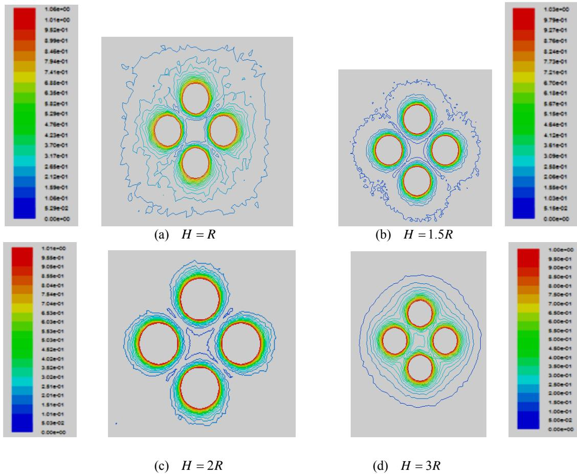
Figure 3. Velocity of ground effect at different altitudes.
