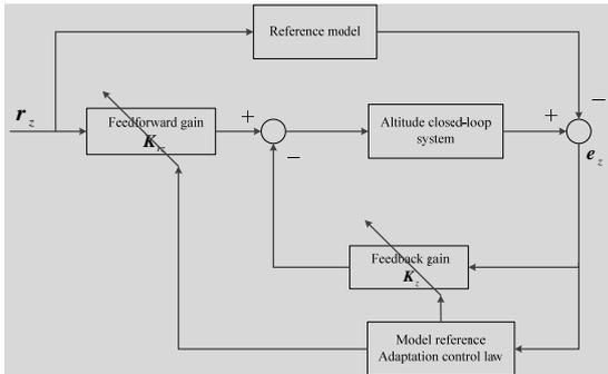
Figure 5. Model reference adaptive control on altitude channel
