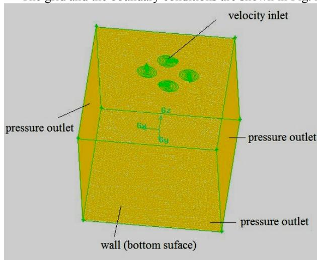
Figure 2. Grid and boundary conditions
