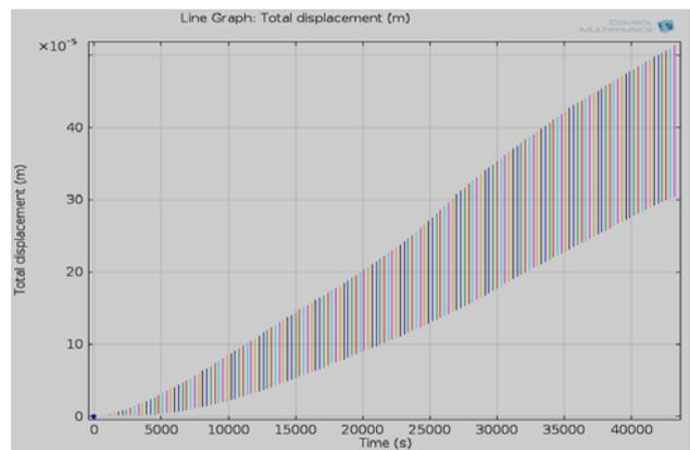
Fig.7 The left boundary displacement change of dinosaur fossils
