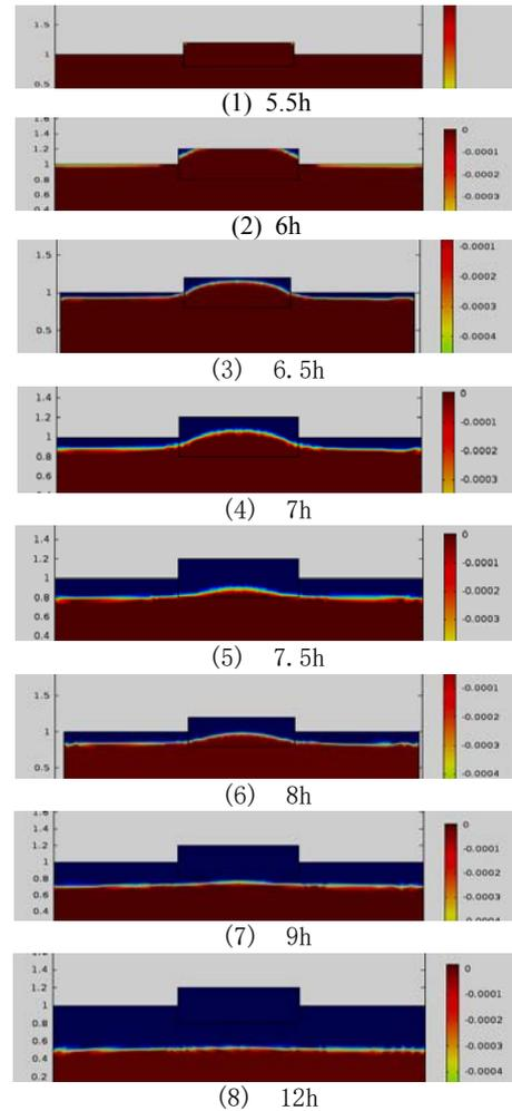
Fig.9 Internal pore water freezing process
