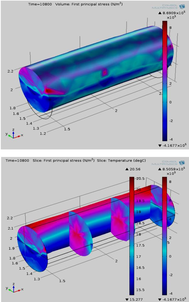
Fig.8 Fossil surface stress distribution and internal stress and temperature slices
