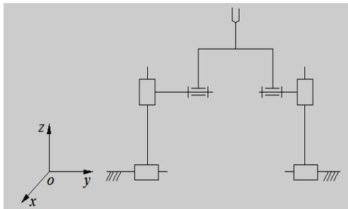
(a) Symmetric parallel mechanism of 4 degree of freedom
