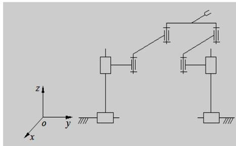
(a) Symmetric parallel mechanism of 5 degree of freedom.
