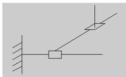
Figure 4. Two orthogonal translation input branch
