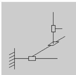
Figure 5. Three orthogonal translation input branch
