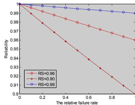
Fig.2 The Changes of the Reliability of the Module with the Relative Failure Rate
