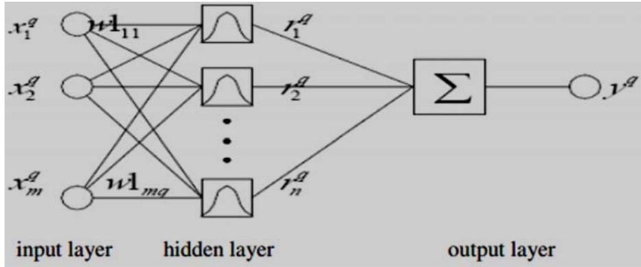
Fig.1 The Structure of RBF Neural Network
