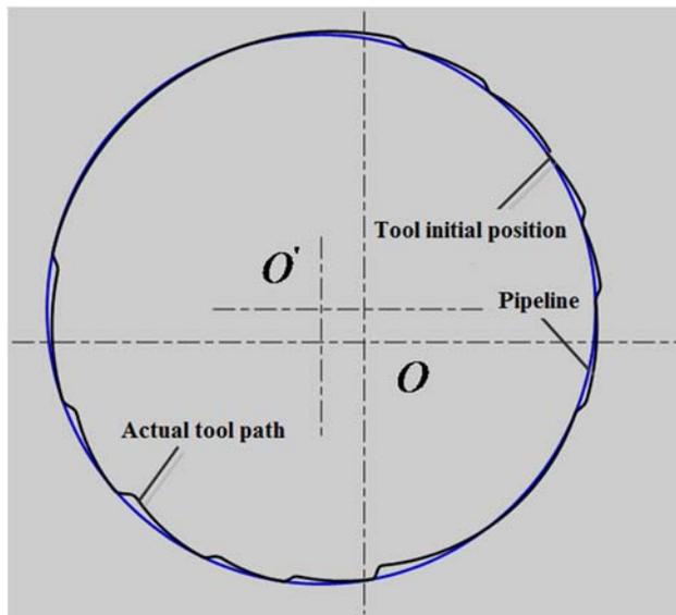
Figure 9. Schematic diagram of inner chamfering tool's error compensation path
