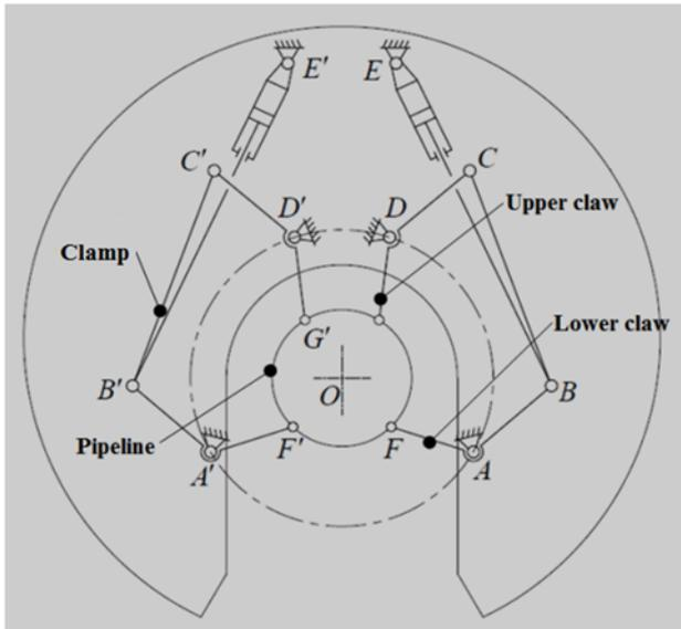
Figure.3. Schematic diagram of the Clamp
