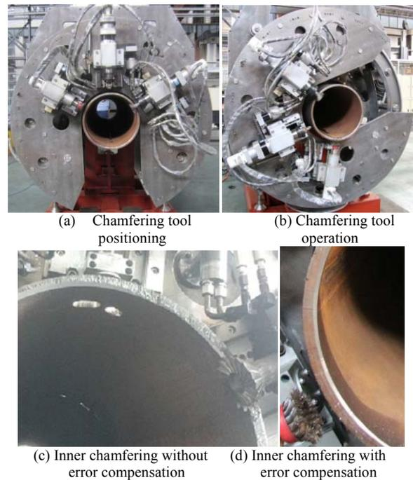
Figure.8. Chamfering experiments
