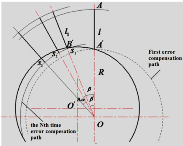
Figure.7. Schematic diagram of tool path error in any position
