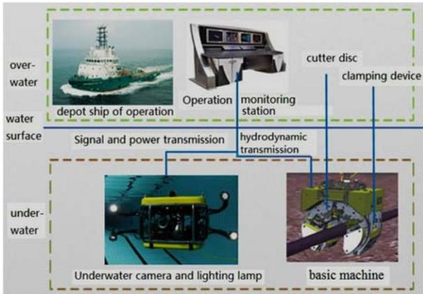
(a) The system of subsea multifunctional equipment.
