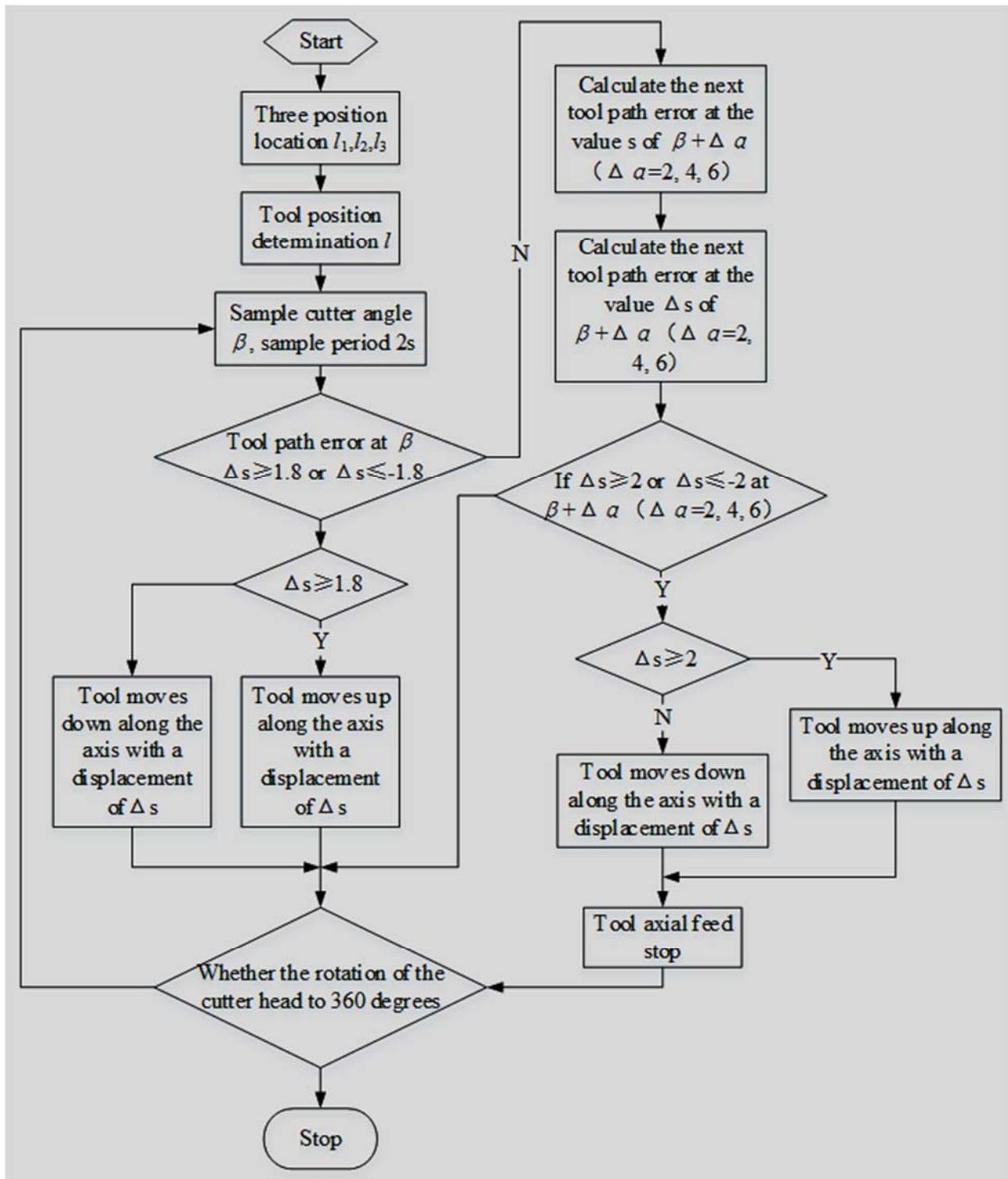
Figure.6. The flow-process of tool path error correction program.
