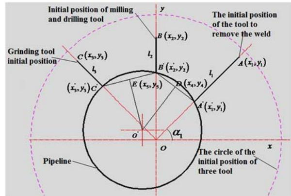
Figure.4. Simplified model of cutter and pipe in the mid-plane of tool
