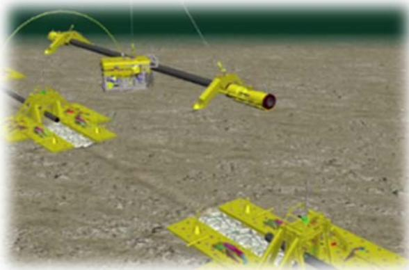
(b) Cutting submarine pipeline and slinging the damaged pipe section
