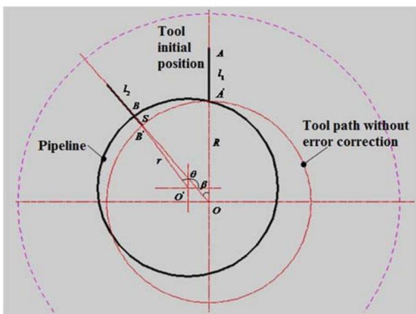
Figure.5. Schematic diagram of tool path model without correction
