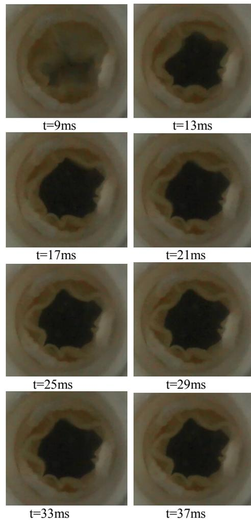
Fig.7 Opening Process of the Valve
