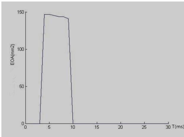
Fig.8 Effective Orifice Area Changes by the Time
