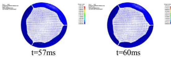
Fig.5 Stress Distribution of the Spherical Leaflets
