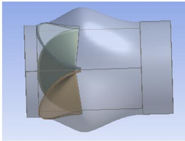
Fig.3 Coupling Model of leaflets and blood
