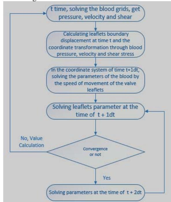
Fig.1 Blood and Leaflets Coupling Calculation Process
