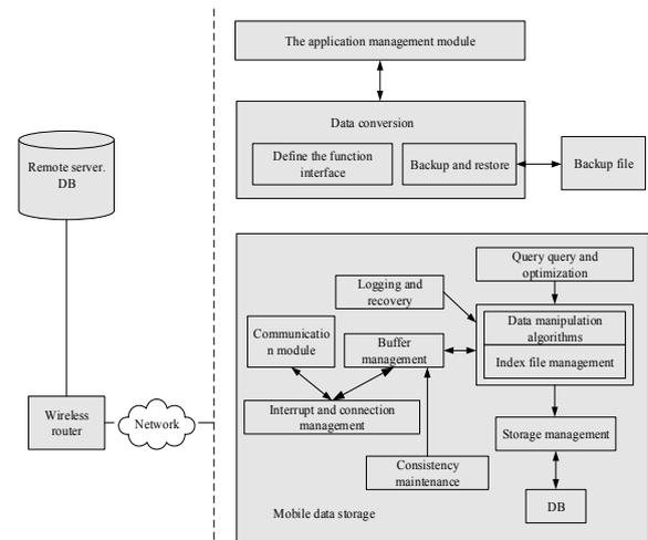
Figure 4. Mobile data storage management model for applications.
