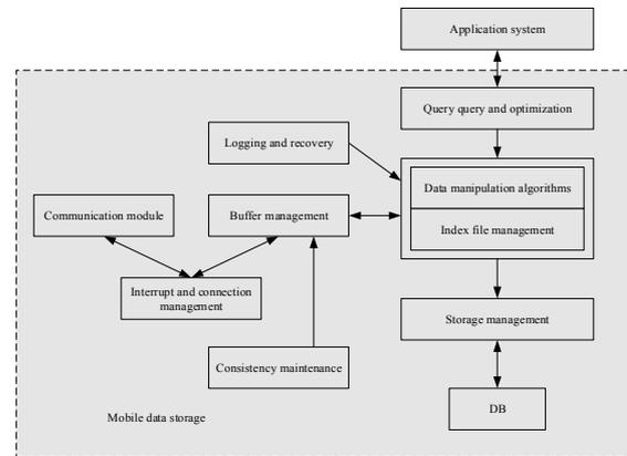
Figure 2. Structure of data management for mobile data storage.
