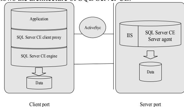
Figure 3. SQL Server CE system structure diagram.
