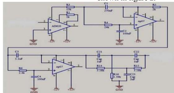
Figure 2. ECG signal conditioning circuit
