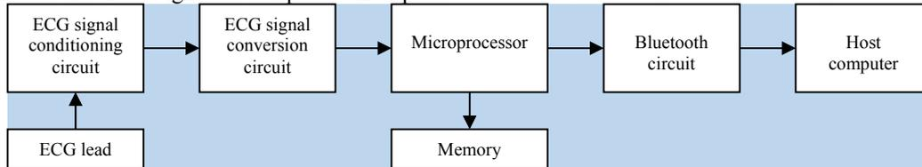
Figure 1. Structure of ECG acquisition system
