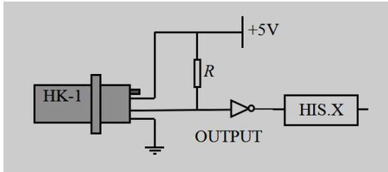
Figure 4. Cylinder detection signal and top center position signal processing circuit
