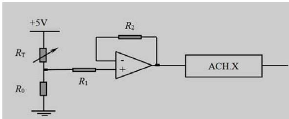
Figure 5. Water temperature measurement circuit
