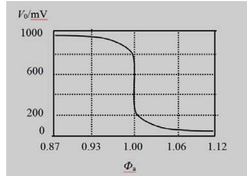
Figure 7. Relationship of air fuel ratio and oxygen sensor output voltage
