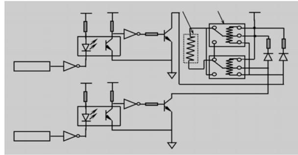
Figure 12. By-pass air valve driving circuit
