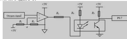
Figure 8. Oxygen sensor signal processing circuit
