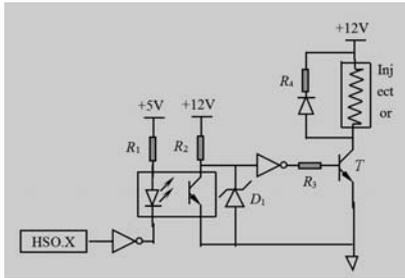
Figure 10. Oil Injector driving circuit
