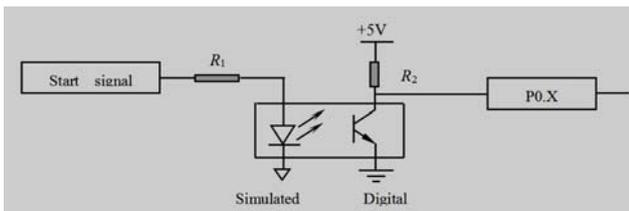
Figure 6. Start signal processing circuit
