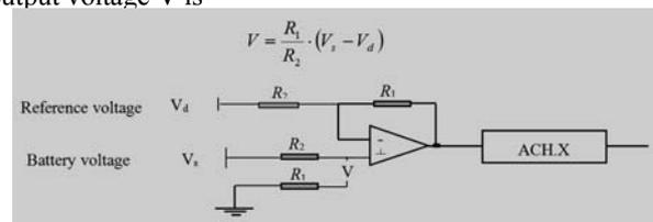
Figure 9. Battery voltage processing circuit
