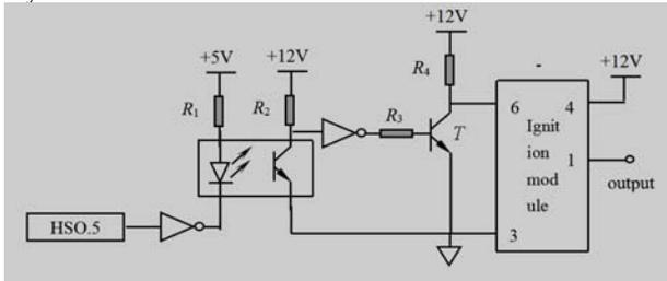
Figure 11. Ignition driving circuit
