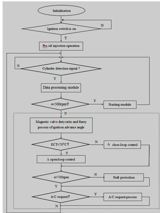
Figure 13. Master control program circuit
