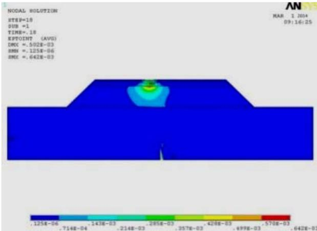
Fig.8 The equivalent strain nephogram in soft pavement
