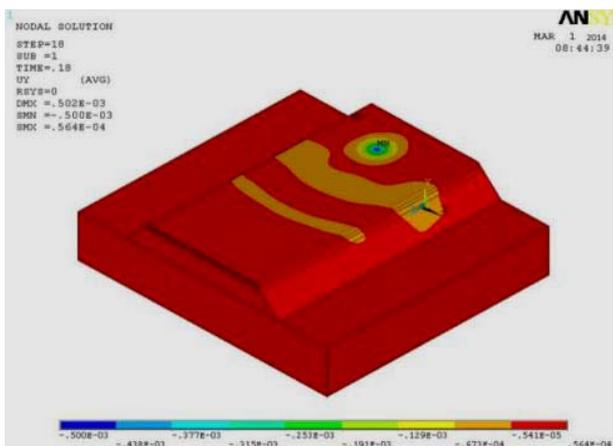
Fig.6 The total vertical displacement in step 18
