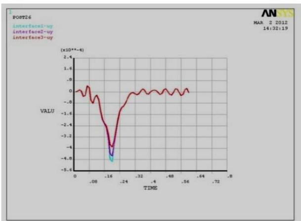
Fig.9 The vertical displacement time-procedure
