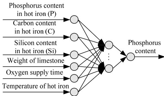
Figure 2. Prediction Model of Phosphorus Content Based on RBF Neural Network
