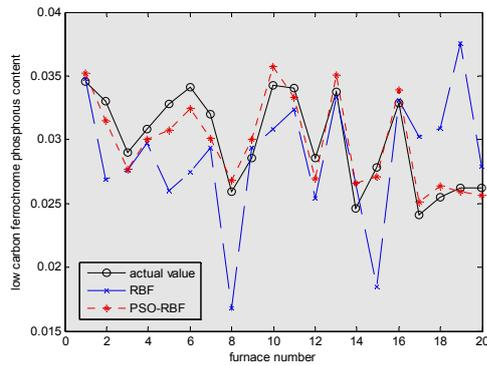
Figure4. Comparison of Forecasting Results of RBF and Modified PSO-RBF Algorithms
