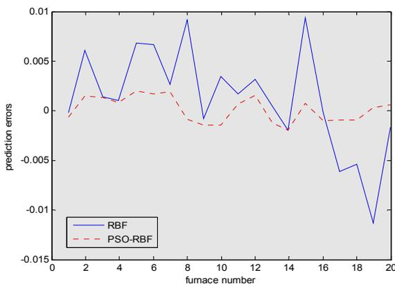
Figure5. Comparison of Prediction Error of RBF and Modified PSO-RBF Algorithms.
