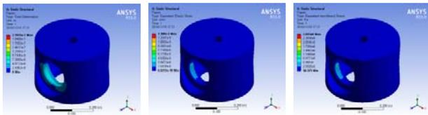
Figure 11 Total distortion, equivalent elastic strain and effective stress of A-axis box before optimization
