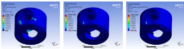
Figure 12 Total distortion, equivalent elastic strain and effective stress of A-axis box after optimization
