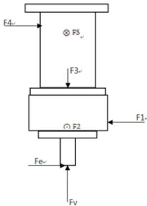
Figure 8 Stress condition of A-axis milling head body
