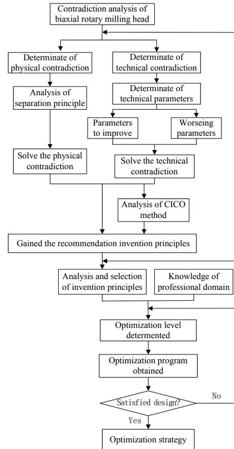
Figure 2. Flowchart for the optimization process of bi-rotary milling head using TRIZ
