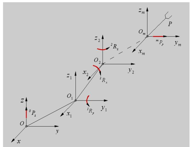
Fig.1 Moving element on serial branch
