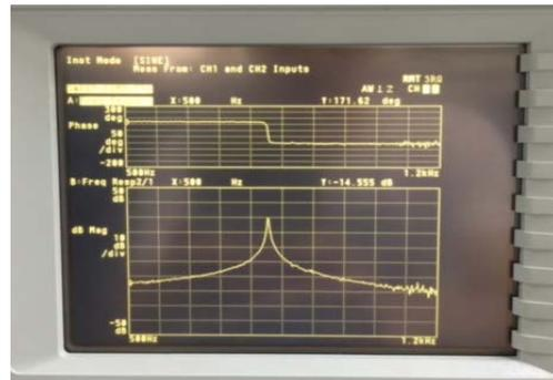
Fig.14 Result of open-loop transfer function
