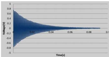
Fig.12 Typical Time-domain oscillation damping curve for Q-value calculation
