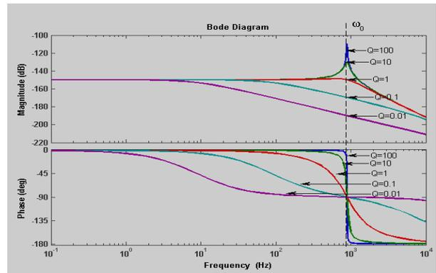
Fig.2 Frequency response of typical 2<sup>nd</sup> order system
