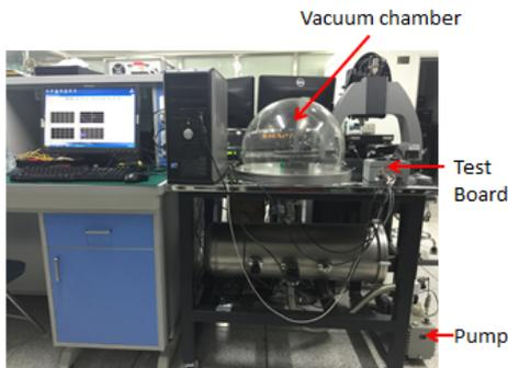
Fig.11 Q-test instrument
