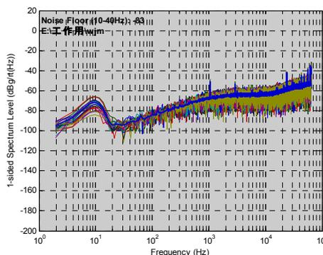
Fig.19 Power spectral density of accelerometer’s noise with non-vacuum sealed device
