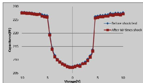
Fig.15 Top Capacitor C-V Curve before and after shock test
