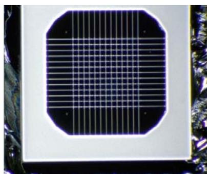
Fig.7 Grooves etched on cap-wafer
