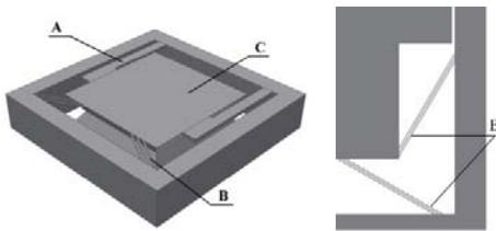
Fig.1 Proof-mass and frame of mechanical device
