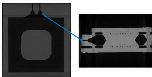
Fig.6 CT image of the vent-hole of the finalized device
