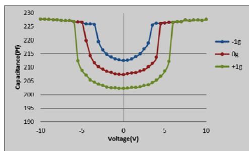
Fig.10 Top Capacitor C-V Curve under -1g, 0g, 1g gravity
