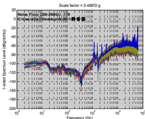
Fig.18 Power spectral density of accelerometer’s noise with vacuum sealed device
