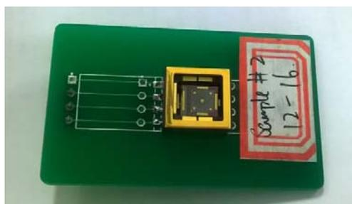
Fig.8 Wire bonded device mounted on PCB board
