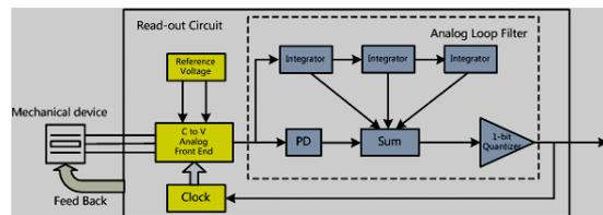
Fig.16 Mechanical device with closed-loop circuit
