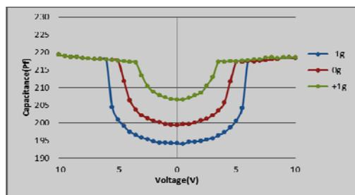
Fig.9 Bottom Capacitor C-V Curve under -1g, 0g, 1g gravity
