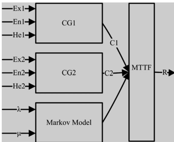
Fig. 4 The Cloud Reliability Estimation Method Diagram
