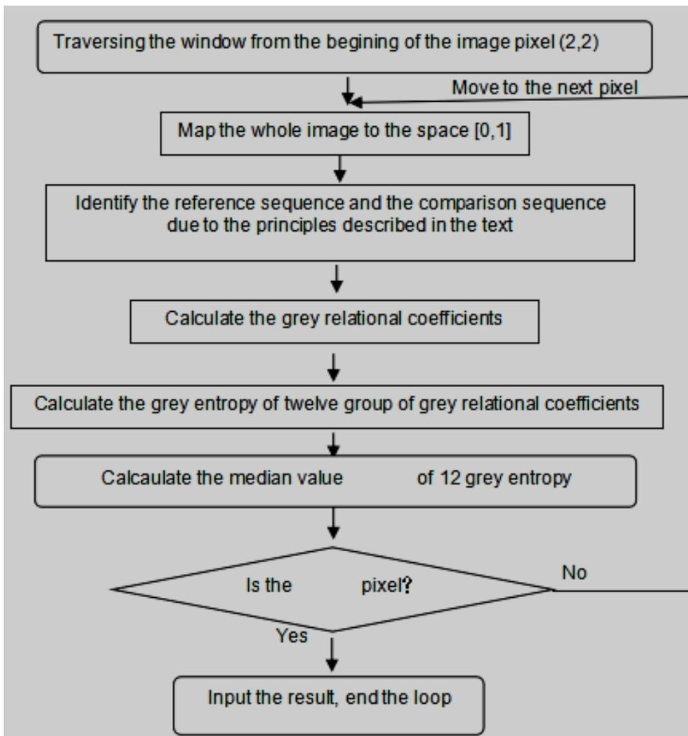
Fig.1 Diagram of grey entropy method
