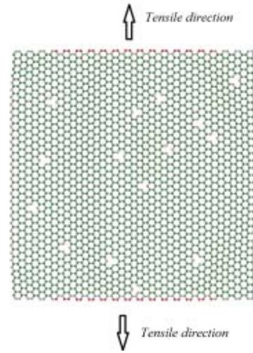
Fig.2. Atomic Configuration Diagram of Tensile Model Irradiated By C Atoms
