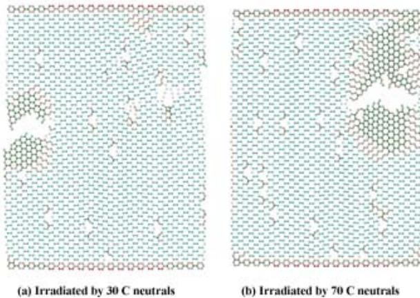
Fig.7. Fracture mode of irradiated graphene
