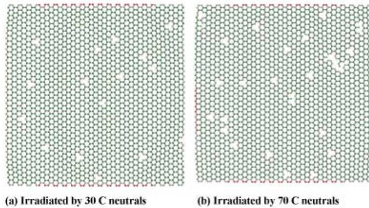
Fig.3. Atomic configuration diagram of gaphene irradiated by 30 and 70 C Atoms
