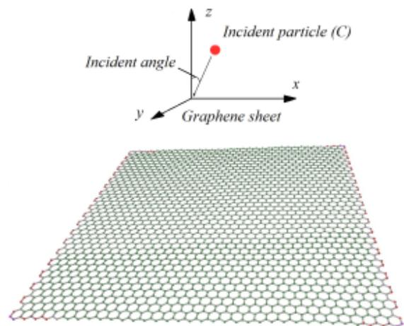
Fig.1. Atomic Configuration Diagram of The Model Irradiated By C Atoms
