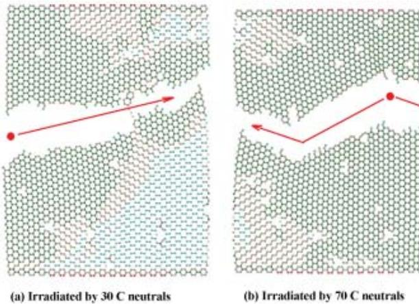
Fig.8. Fracture propagation (dot represents the fracture starting point, arrow represents fracture direction)
