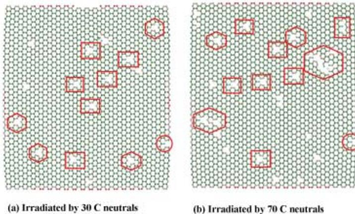
Fig.4. Atomic configuration diagram of extension of defects at the edge
