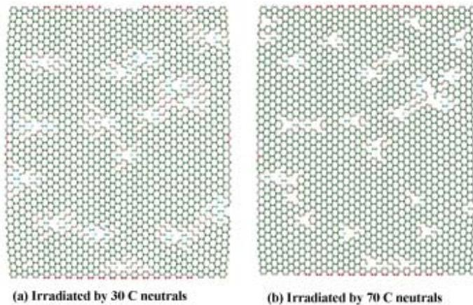
Fig.5. Adjacent defect regions interconnect and form defect clusters
