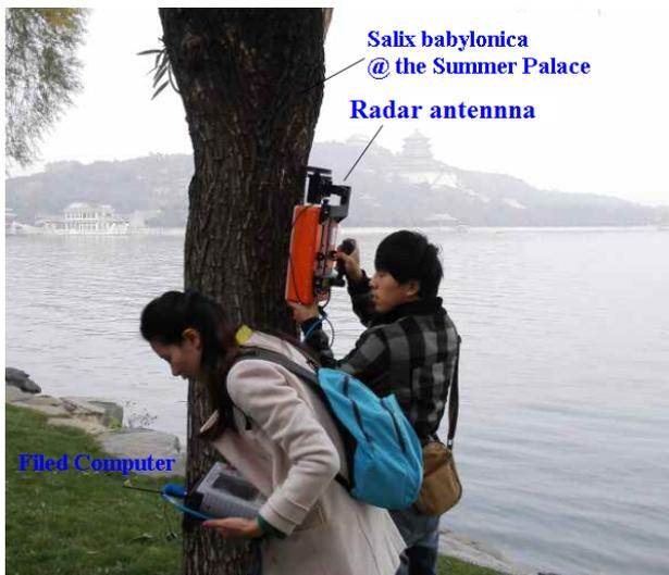
Fig. 2. Filed Experiment at the Summer Palace, Beijing, China, using Tree radar system with 900MHz GPR antenna
