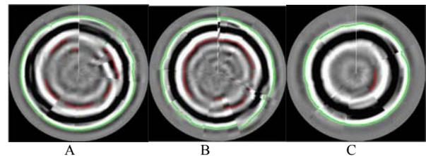
Fig. 5. Gray scale detection of selected specimens, A is 1# B is 2# C is 3#
