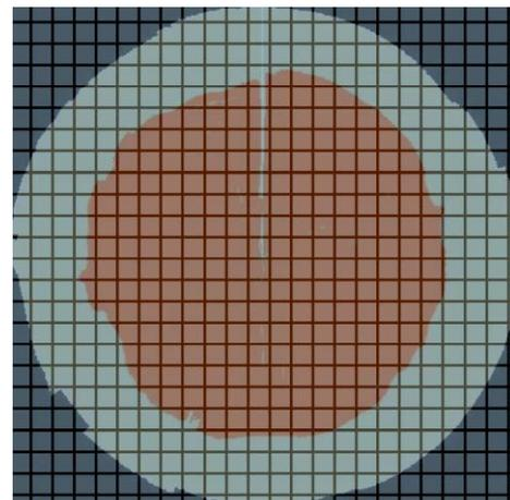
Fig. 6. Diagram of coordinate paper method for measuring defect area, 314 grids is decay area shown in red and 803 grids is total area of trunk; ratio of decay area to trunk area is 39.1%
