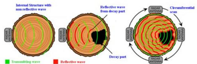
Fig. 1. Circumferential scanning wooden structure using radar wave
