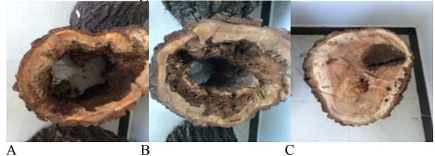
Fig. 4. Selected willow trunk specimens with different levels of defects, A is 1# B is 2# C is 3#
