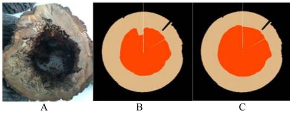
Fig. 6. Compared result of actual defect (shown in A) with detected defect without model correction (shown in B) and with model correction (shown in C) for 1# specimen
