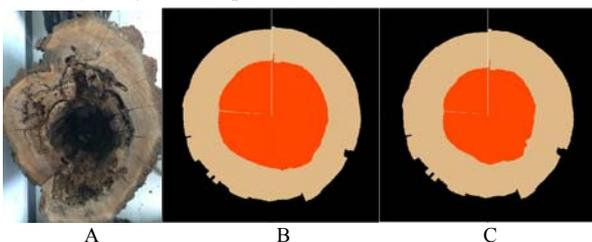
Fig. 7. Compared result of actual defect (shown in A) with detected defect without model correction (shown in B) and with model correction (shown in C) for 2# specimen
