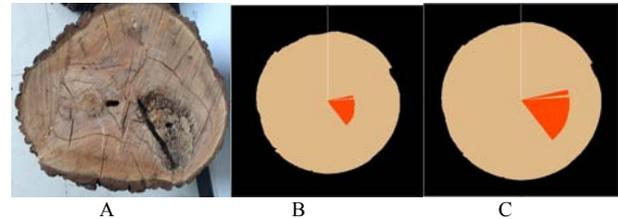
Fig. 8. Compared result of actual defect (shown in A) with detected defect without model correction (shown in B) and with model correction (shown in C) for 2# specimen
