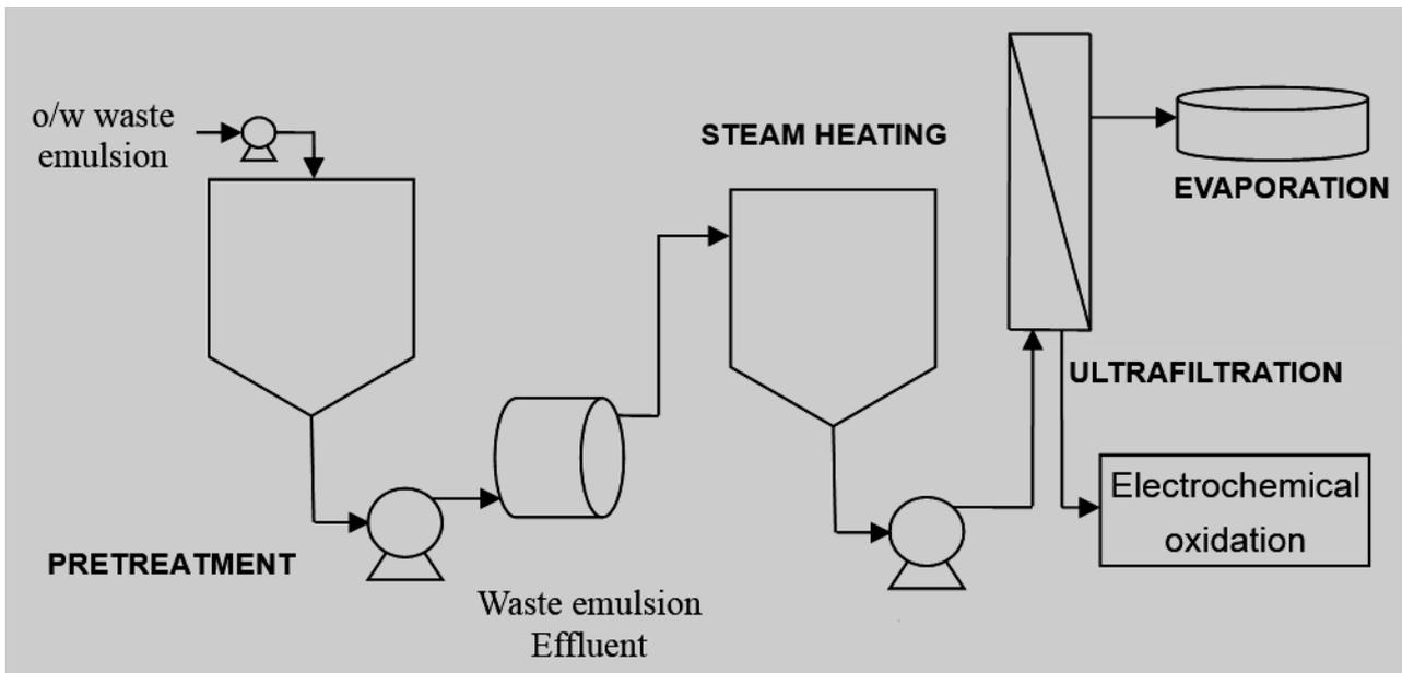
Fig.(3). Schematic Diagram Of The Proposed Of UF And Electrochemical Oxidation For The Treatment Of Waste O/w Emulsions.
