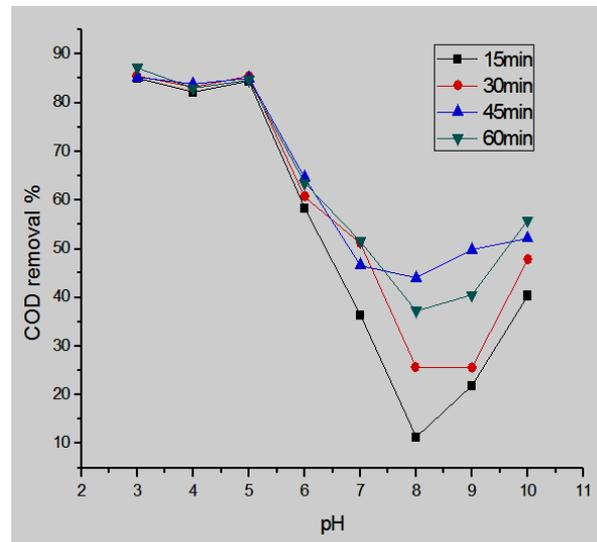
Fig.(8). Effect Of pH On COD Removal Efficiency
