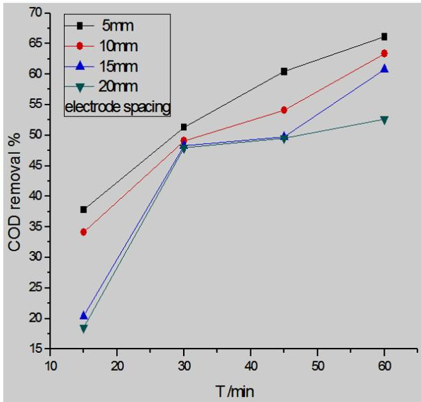
Fig.(7). Effect Of Electrode Spacing On COD Removal Efficiency
