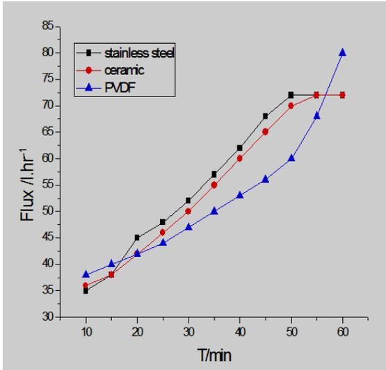
Fig.(4). The Flux vs.Time Of Three Series UF Membranes Run Before Pretreatment.
