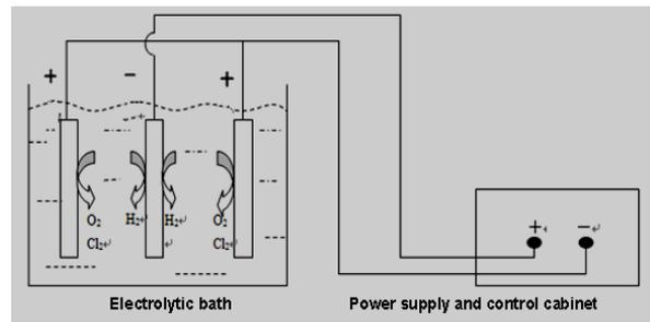
Fig.(1). Electrochemical Oxidation Experimental Schematic
