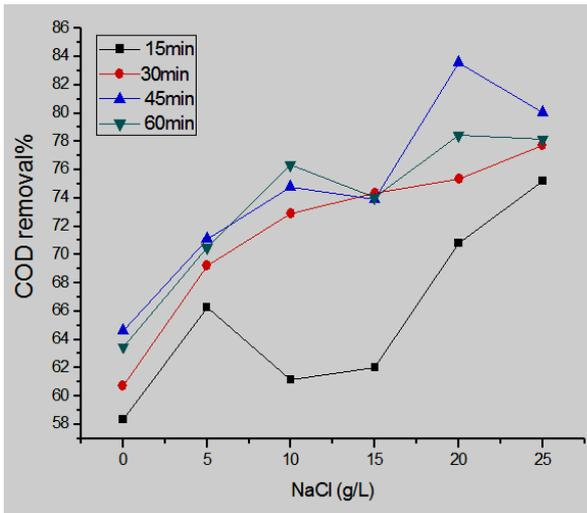
Fig.(9). Effect of fortified concentration of NaCl
