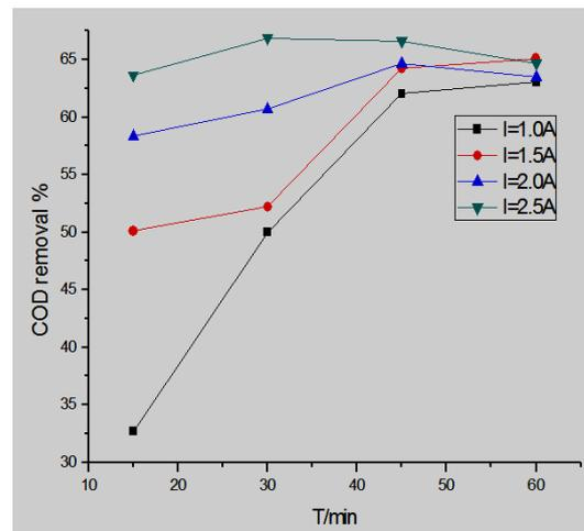
Fig.(6). Effect Of Current Density On COD Removal Efficiency
