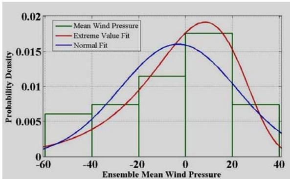
Fig. (4). Histogram of Wind Force Acted on Ballast Effective Surface.
