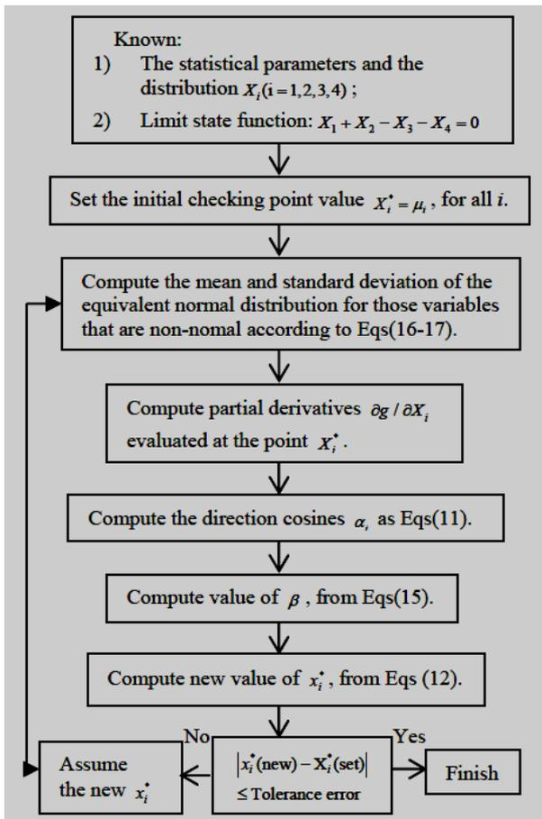
Fig. (6). Iteration Computing Process of the Reliability Index.
