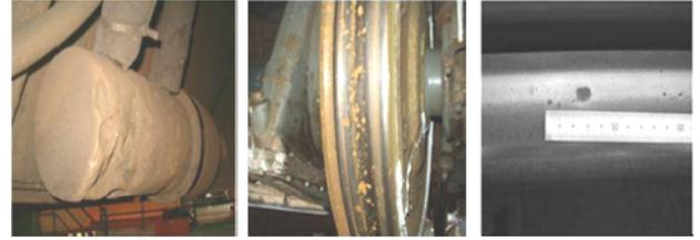
Fig. (1). Ballast Flying Damage
