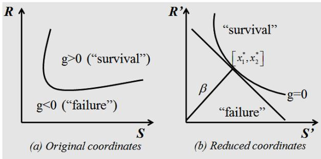
Fig. (5). Formulation of Safety Analysis in Original and Reduced Variable Coordinates
