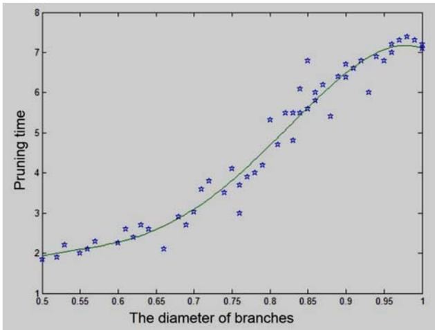
Fig. (4). The figure reflecting the changes between different diameters and different cut time of branches.
