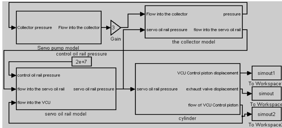
Fig.2: the simulation block diagram of the servo oil common rail system.
