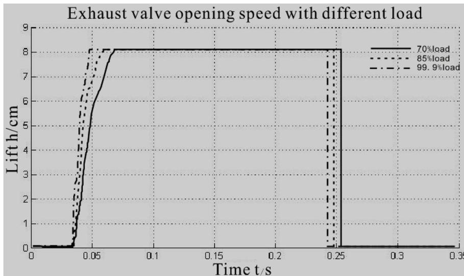
Fig.10: the effect of various diesel loads on the open speed of exhaust valve
