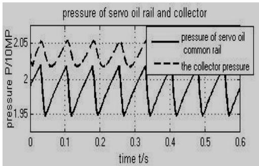
Fig.4: the pressure simulating diagram of the collector and the servo oil common rail.
