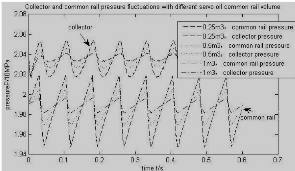
Fig.8: the impact of the volume of servo oil common rail on the pressure stability
