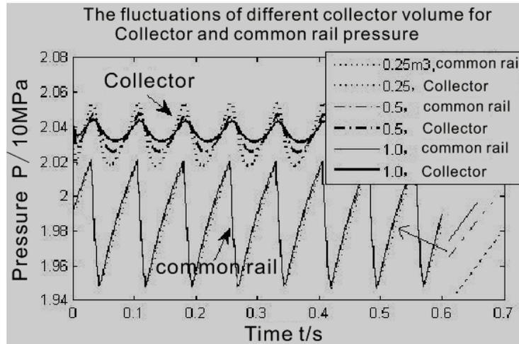
Fig.7: the impact of collector volume on the pressure stability
