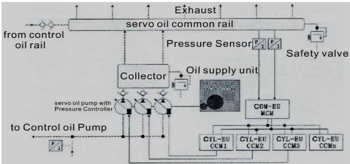
Fig.1. The principle of servo oil common rail system
