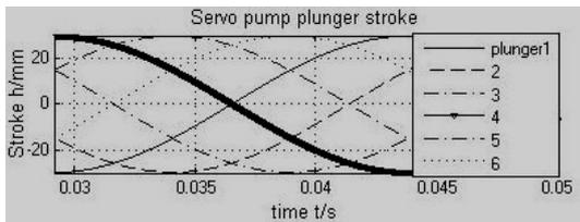
Fig.3: simulating curve of the servo pump plunger displacement.
