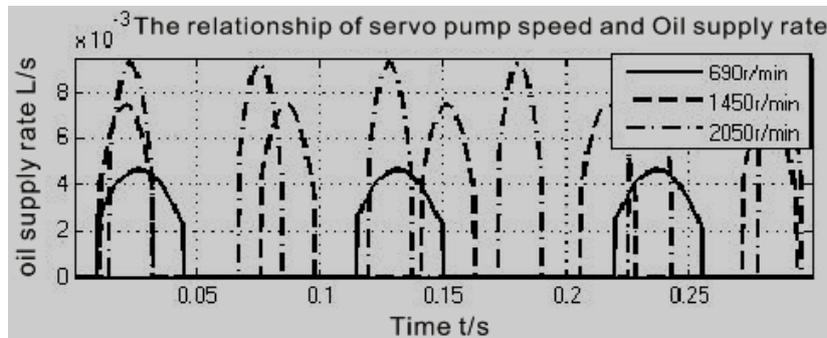
Fig.6:the relationship between servo oil pump speed and the oil supply rate
