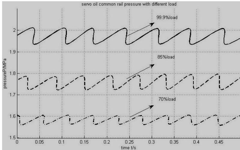
Fig.9: the effect of load on the pressure fluctuation of servo oil common rail
