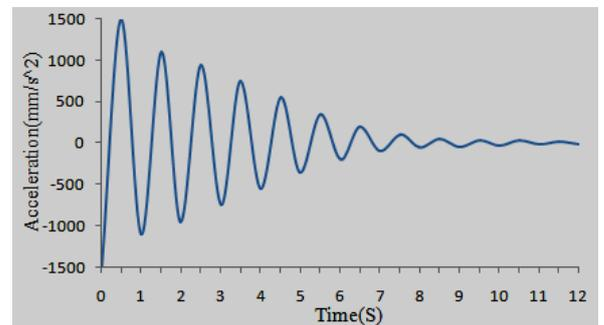
Fig. (3). The Time-varying Curve of the Acceleration of the Mass centre of the Optimized Power Assembly along Z Axle Direction Under Idling Condition
