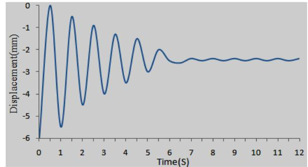
Fig. (2). The Time-varying Curve of the Displacement of the Mass Center of the Optimized Power Assembly along Z Axle Direction Under Idling Condition
