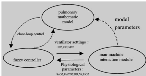
Fig. (1). The Structure of the System
