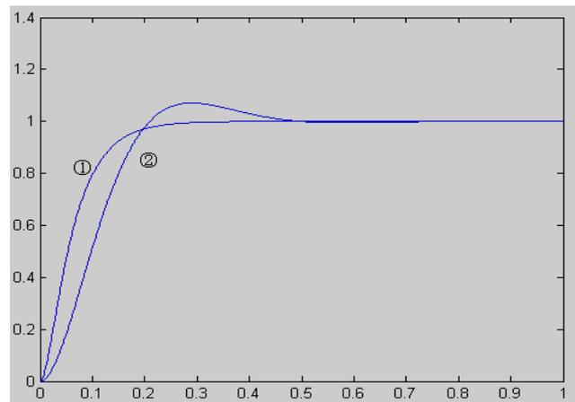
Figure 5 Simulation of fuzzy PID and conventional PID control system
