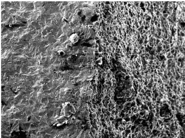
Fig.2 SEM image of 2# sample of side fracture morphology SEM scanning
