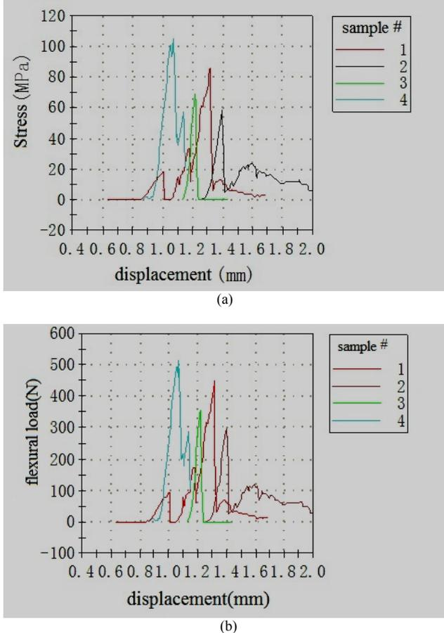
Fig.5 The relationship of the stress and bending load with the displacements.
