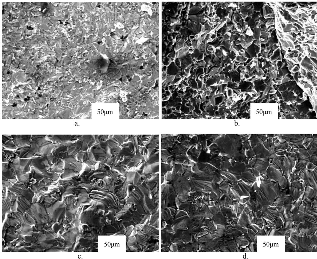
Fig 1. Microstructures of TiC-based cermets with different contents of Mo by SEM: (a) Ti/Mo=0.9:0.1; (b) Ti/Mo=0.8:0.2; (c) Ti/Mo=0.7:0.3; (d) Ti/Mo=0.7:0.3
