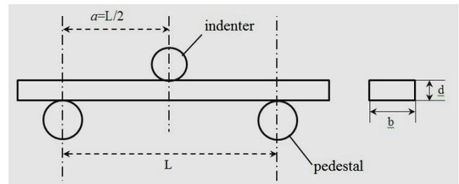
Fig. 4 Bending strength test structure diagram.
