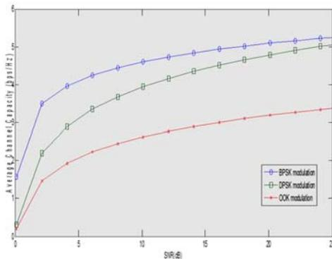
Figure 5. Channel capacity vs SNR
