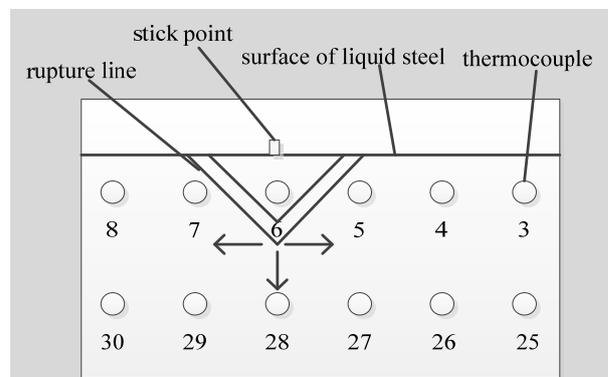
Figure. 2 The model of sticking breakout.
