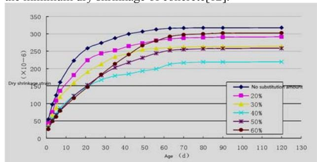
Figure 11. Relationship curves between dry shrinkage strain and age
