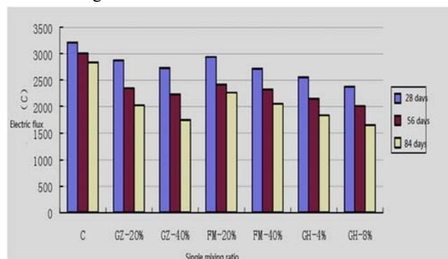
Figure 8. The relationship between concrete electric flux and age mixing admixture
