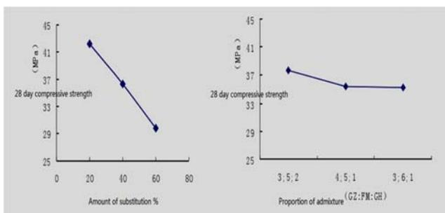
Figure 7. Effect of substitution amount and blending ratio on compressive strength of 28 days
