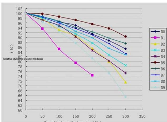
Figure 10. Relative dynamic modes of concrete after freeze-thaw cycles
