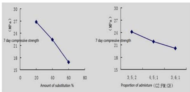
Figure 5. Effect of substitution amount and blending ratio on compressive strength of 7 days
