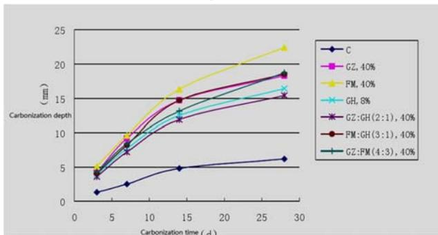
Figure 9. Carbonation curves of single and double admixtures concrete
