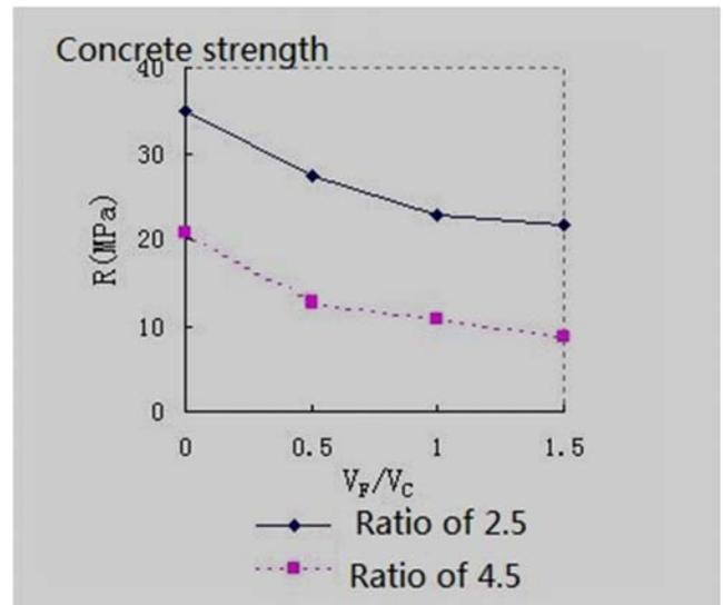
Figure 2. Schematic diagram of effect of pozzolanic effect on concrete strength.
