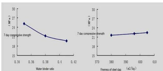
Figure 6. Influence of water binder ratio and steel slag fineness on compressive strength of 7 days
