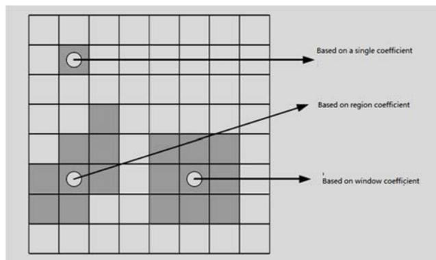
Figure 2. Schematic diagram of classification of image fusion rules
