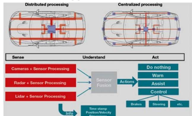
Figure 6. Schematic diagram of multisensor data fusion algorithm
