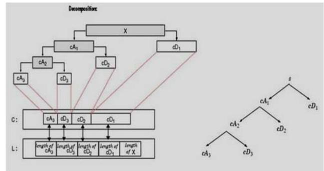
Figure 4. Mallat Algorithm Working Schematic Diagram
