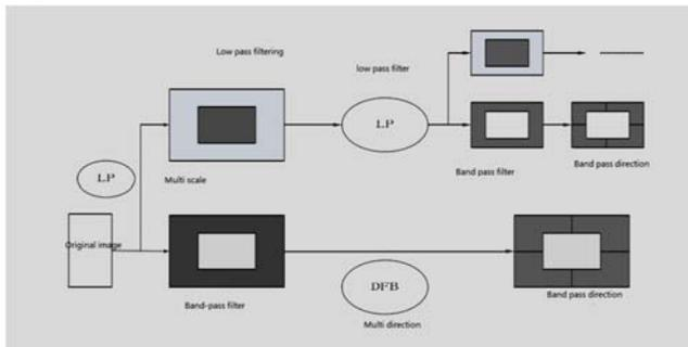
Figure 7. Schematic diagram of Contourlet transform decomposition process
