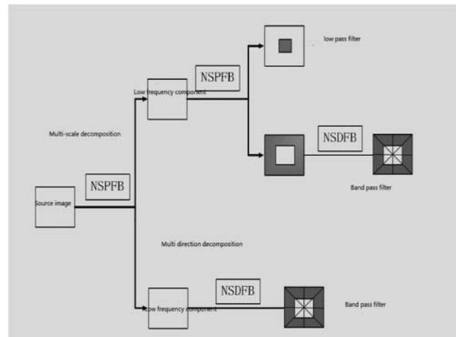
Figure 9. Schematic Diagram of NSCT Algorithm Image Fusion
