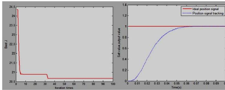
Figure 2. SGA PID parameters to achieve the online tuning and PID controller emulator
