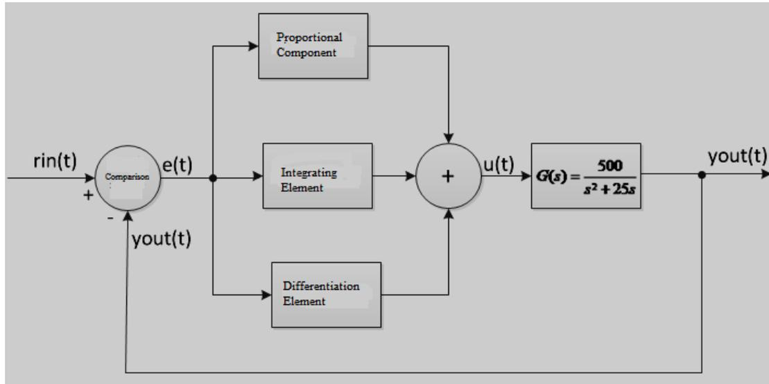
Figure 1. Block diagram of a level control system of FIG.
