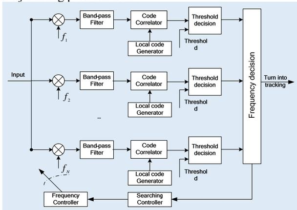
Figure2. Parallel sliding correlation acquisition diagram.
