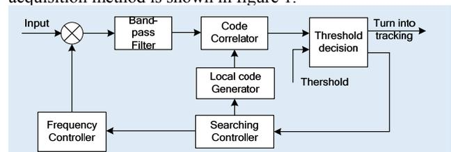
Figure 1. Serial sliding correlation acquisition diagram
