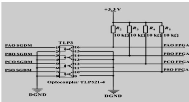
Figure 4. FPGA input signal
