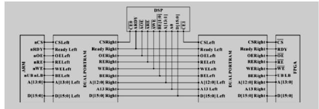
Figure 2. ARM, DSP, and FPGA interface circuit
