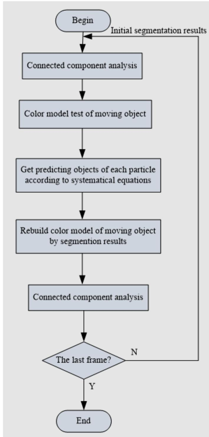
Fig. (2). Flowchart of Post-processing
